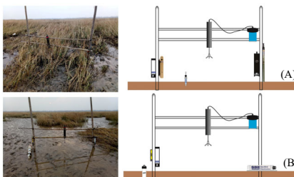
Fig. 2 Schematic figure of instruments used in This study and their deployment height located at the surface sediment. (A) Saltmarsh station (B) Tidal flat station
